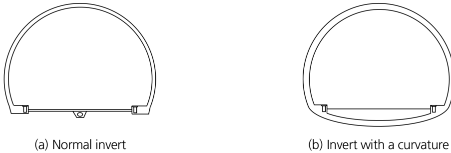
Fig. 1. Tunnel invert with a curvature
